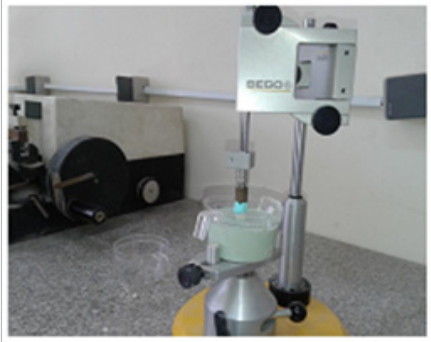
Figure 1: Milling surveyor used to mount the tooth in the mold.
