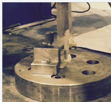
Figure 1: A representative sample loaded in the jig of the SBS testing machine.
