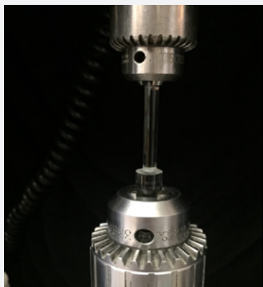
Figure 2: The gap was adjusted at 1mm using the crosshead controller and the excess of composite was cleaned off.
