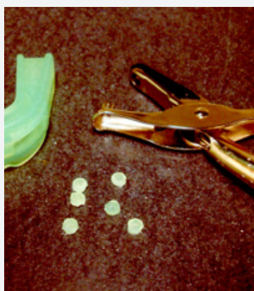
Figure 1: Discs Were Prepared from Night Guard. A standard hole puncher was used to make circular discs from a hard-soft acrylic mouth guard. Disc sizes were approximately 6mm wide in diameter and 2.5mm thick.
