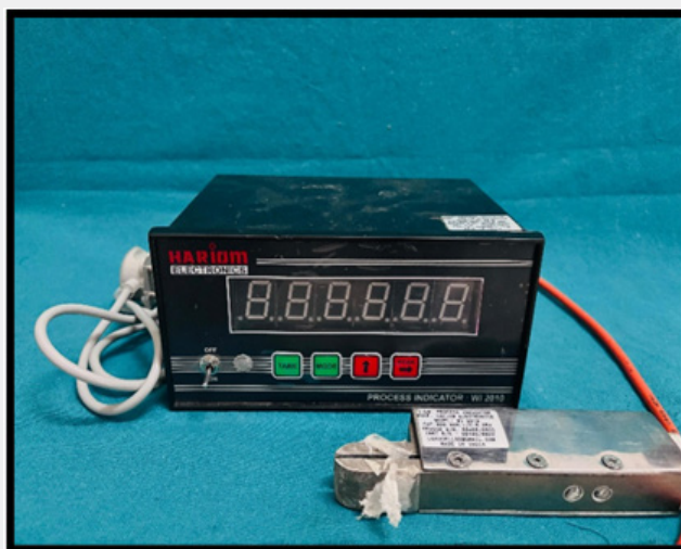
Figure 2: Occlusal Bite Force Metre with Bite Force Sensor.
