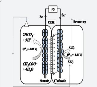
Figure 1: Electro-methanogenesis process in BES having biotic anode and cathode.
