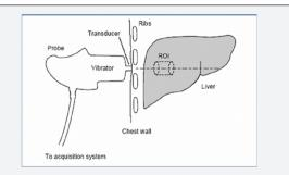
Figure 1: Schematic representation of principle of Transient Elastography.
