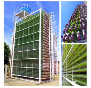
**Figure 1:** Compact photobioreactor for microalgae cultivation built at UFPR.
