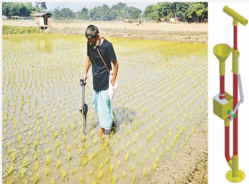
Figure 3: Working with USG deep placement injector.
