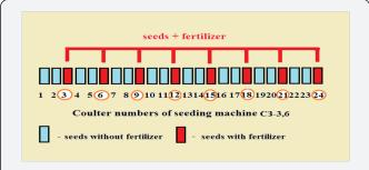
**Figure 1:** The scheme of regulation of coulters of the SZS-3.6 drill for partial separation of seed flows during sowing.
