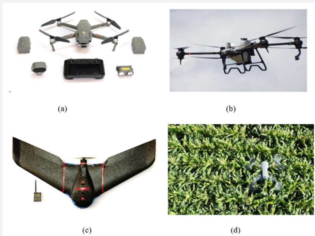
Figure 1: (a) Multirotor for scanning; (b) Multirotor for product application, Hexacopter; (c) Fixed Wing, Fixed-wing (eBee); (d) Multirotors.
