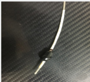
Figure 2a: Stethoscope Ear piece as source carrier with polyethylene catheter.
