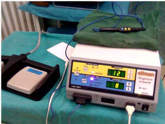
Figure 1: Ellman Surgitron 4.0 Dual RF, patented by Ellman International Company, Oceanside, New York, USA. Inventor dr Jon C. Garito, Patent reference number# 5.954.686. USA. This was the worlds first discovery of the 4 Mhz Radiofrequency device.
