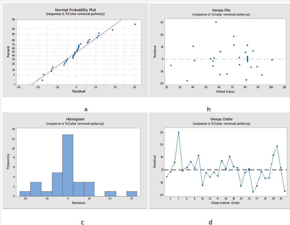
Figure 6: Residual plots for % color removal potency of RR120 (a) Normal probability plot (b) Residual versus fitted values (c) Histogram (d) Residual versus observation order.
