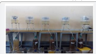
Figure 1: 1 liter digesters with manometer set-up.
