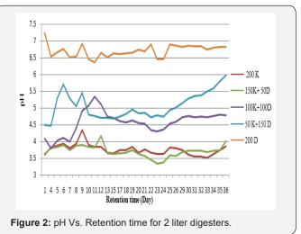
pH drop in anaerobic digestion indicates that acidic intermediates such as VFA are produced in considerable quantities. Lower the pH higher would be the VFA accumulation, which can lead to inhibition of the biogas production during methanogenesis, so a constant pH has been maintained [11-12].
