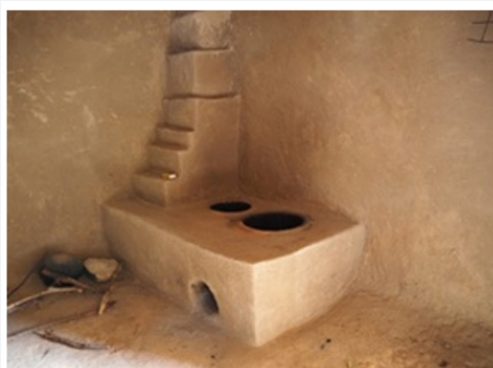
Plate 5: Technological design of ICS; two potholes, well controlled fire chamber.
