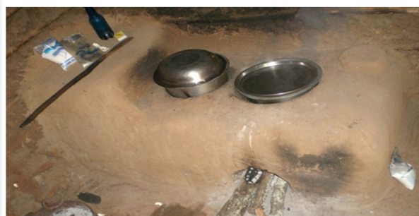
Plate 3: ICS; the technological design dictates efficiency on firewood usage.
