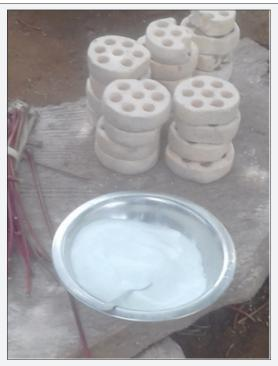
Figure 4: Broken bottles grounded into powder to be baked into beads [5].
