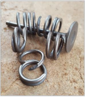
Figure 5: A motor-bike valve and broken springs [7].
