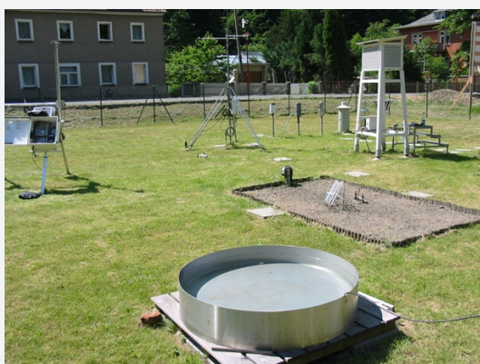
Figure 3: Standard Class-A evaporation pan at Tharandt Met. Station (Photo source: IHM, TU Dresden).
