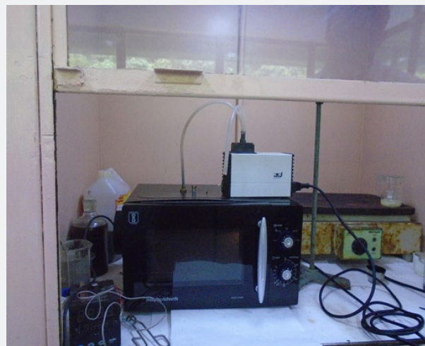
Figure 1: Microwave heating setup in fume hood.
