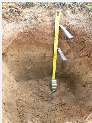
Figure 6: Soil profile at site B showing the restrictive layer richer in iron at a depth between 8 and 23cm (photo by Y. Périard)
