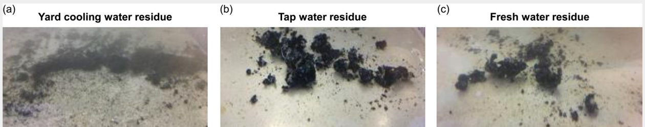
Figure 14: Debris based on the reaction of molten slag to cooling water.
