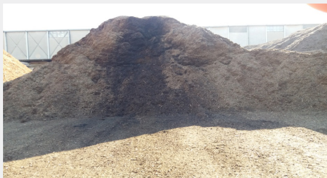
Figure 1: Biomass collection where the zone of the pile heated by air circulation is observed.
