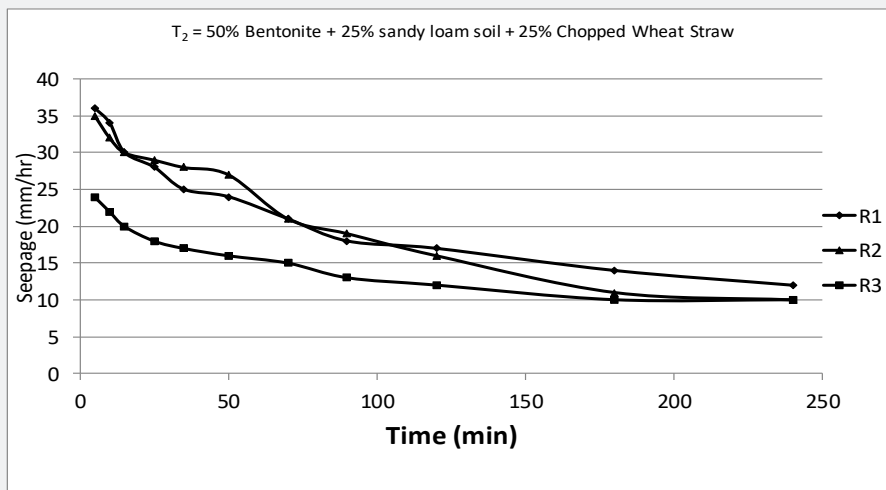
Figure 9: Seepage rates observed over time for the experimental pond (T 2 ).
