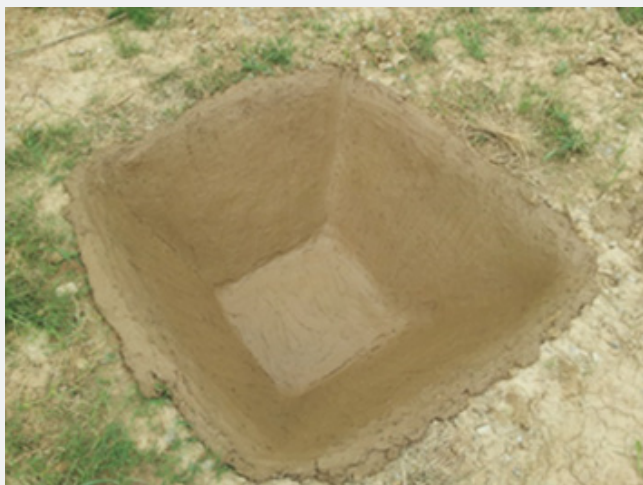
Figure 3: A view of the experimental earthen pond with treatment layer prior to experiment.
