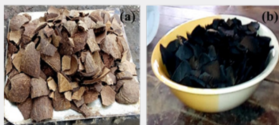
Figure 1: Activated carbon preparation (a) coconut shells (b) carbonized coconut shells.
