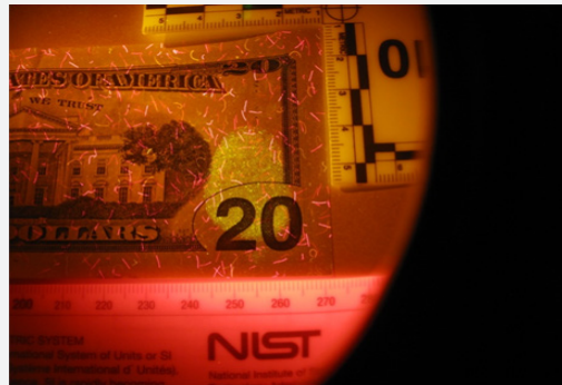
Figure 5: A latent fingerprint (a whorl pattern) with a high-level quality can be clearly observed on the $20 backside after the laser application and photographed under the orange/red filter.
