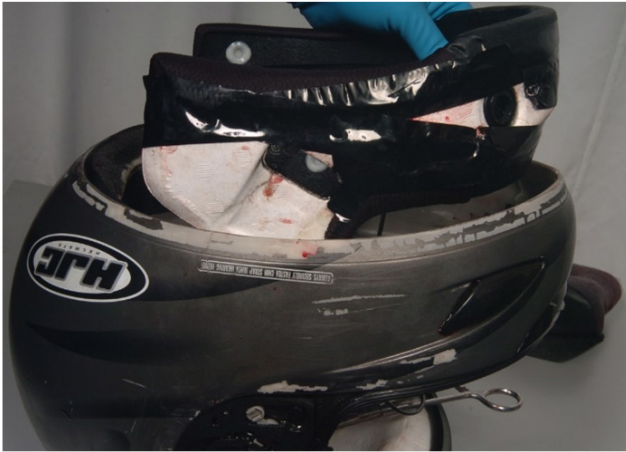
Figure 2: Matching left impact liner damage with the left temporal bone fracture.
