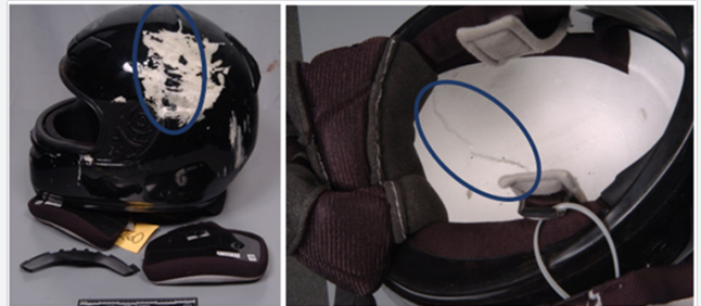
Figure 4: Damage to the left helmet shell and impact liner.
