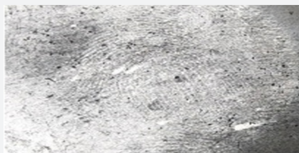
Figure 7: Development Using black Powder after 11 days in fresh water.
