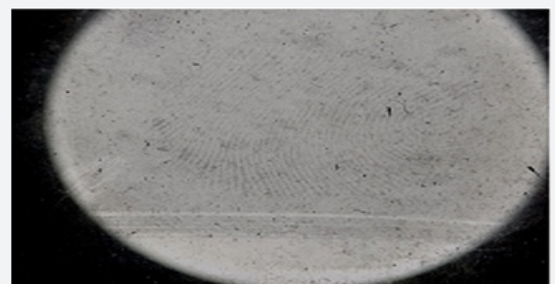
Figure 25: Development Using Cyanoacrylate after 24 hrs in salt water.
