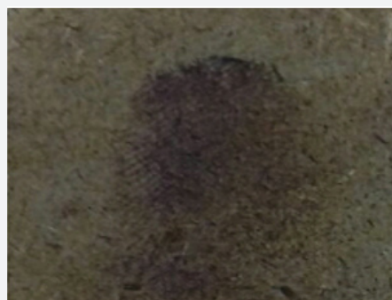
Figure 49: Development Using Iodine fuming after 24 hrs in fresh water.
