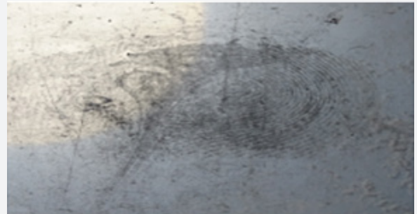
Figure 39: Development Using Black powder after 13 days in fresh water.
