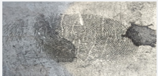
Figure 33: Development Using Black powder after 24 hrs in fresh water.
