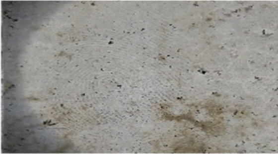
Figure 30: Development Using Cyanoacrylate after 11 days in salt water.
