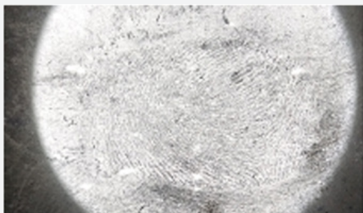
Figure 3: Development Using black Powder after 3 days in fresh water.
