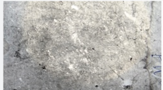
Figure 40: Development Using Black powder after 15 days in fresh water.
