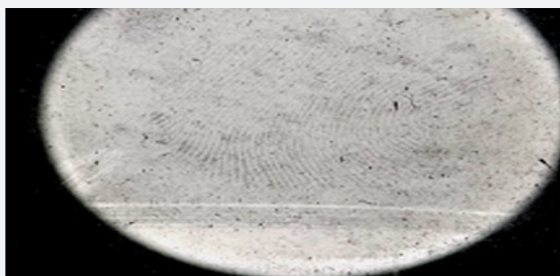
Figure 26: Development Using Cyanoacrylate after 3 days in salt water.
