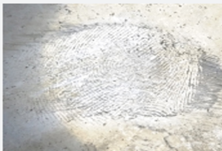
Figure 22: Development Using Cyanoacrylate after 11 days in fresh water.
