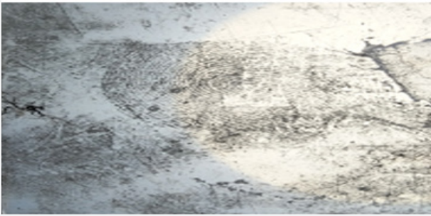
Figure 35: Development Using Black powder after 5 days in fresh water.
