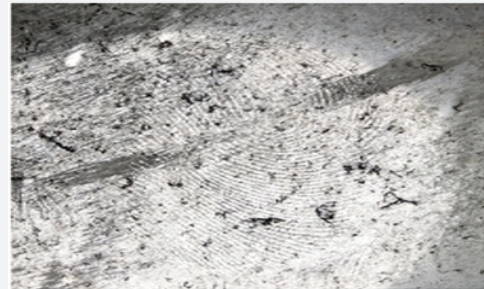
Figure 16: Development Using black Powder after 13 days in Salt water.
