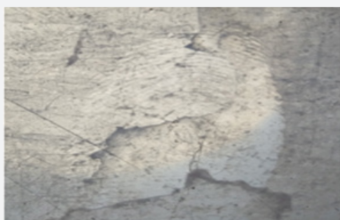
Figure 46: Development Using Cyanoacrylate after 11 days in fresh water.
