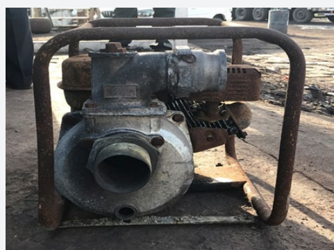
Figure 4: View of centrifugal pump used for refueling.
