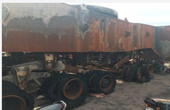
Figure 3: Burnt tires of the crane.
