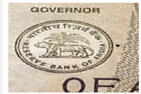
Figure 11: Optical variable ink is used in RBI logo which changes colour from green to blue when the note is tilted.
