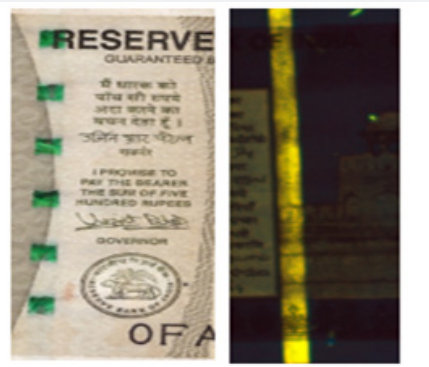
Figure 10: Security thread with 6 inscriptions optical variable ink are used to a color changing from green to blue when the note is tilted and under UV light show full security thread in yellow color.
