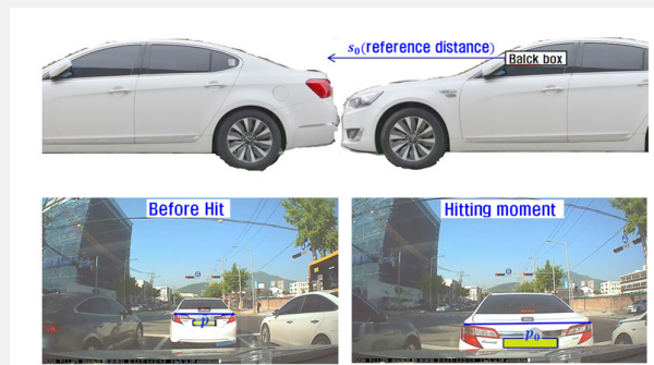
Figure 4: Method of measuring a vehicle's distance from the vehicle ahead of it filmed by the black box.
