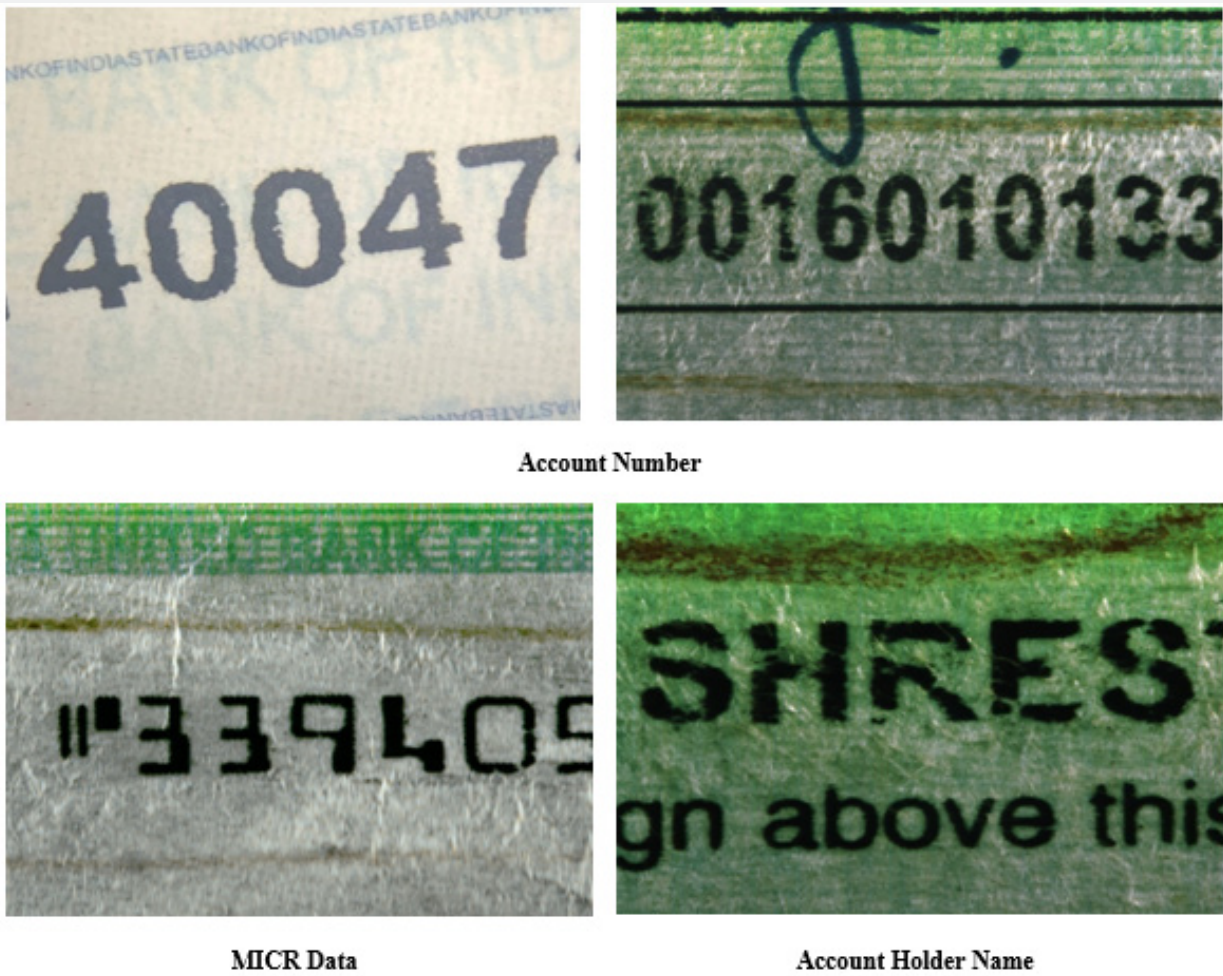
Figure 13: The non-disturbance of fugitive ink in the forged cheques while paper fibres are disturbed during the tampering of the cheques.
