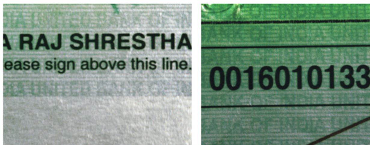
Figure 9: Surface of paper; all fibres are intact with surface with clear texture.
