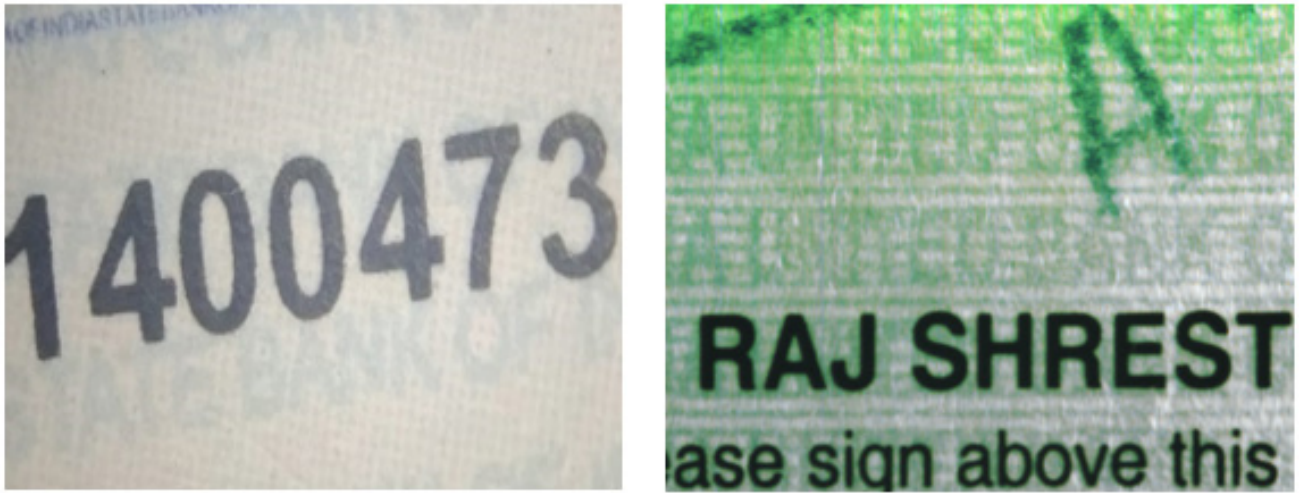
Figure 12: Fugitive ink used for background printing of the genuine cheques. All background printings are distinct and intact in nature.
