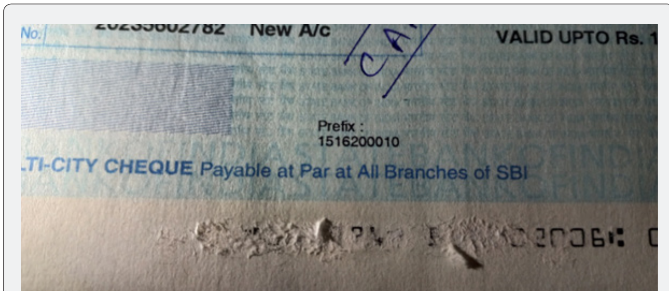
Figure 6: Disturbance of paper fibres using the process of tape lifting easily detected under Side-Light arrangement.
