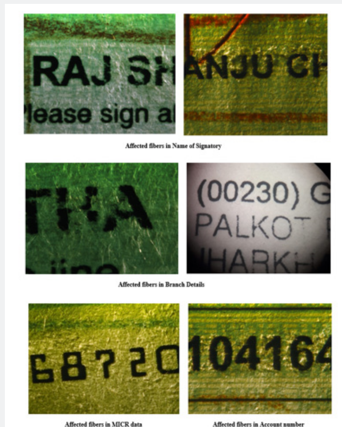
Figure 10: Fibre disturbances at places and toner breaks found under sidelight arrangement in forged cheque.
