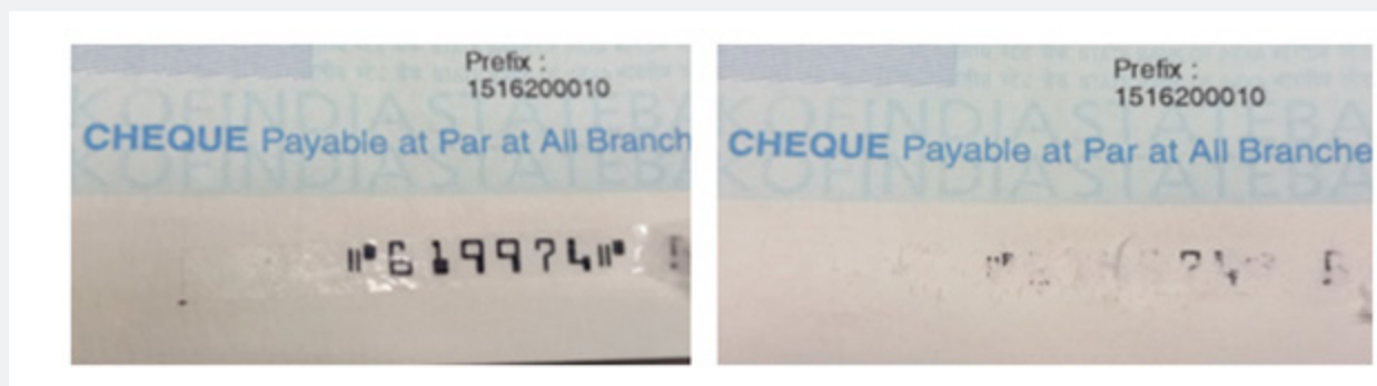
Figure 5: Disturbance of paper fibres using the process of tape lifting.
