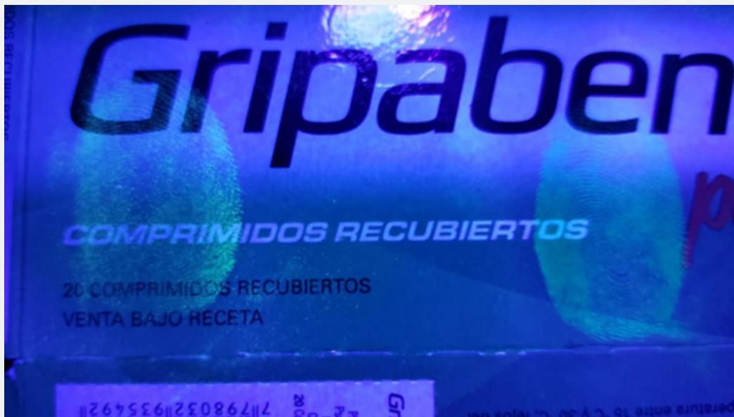
Figure 17: Fingerprints developed with phosphorescent powder (left) and with fluorescent powder (right), without using ultraviolet filters.
