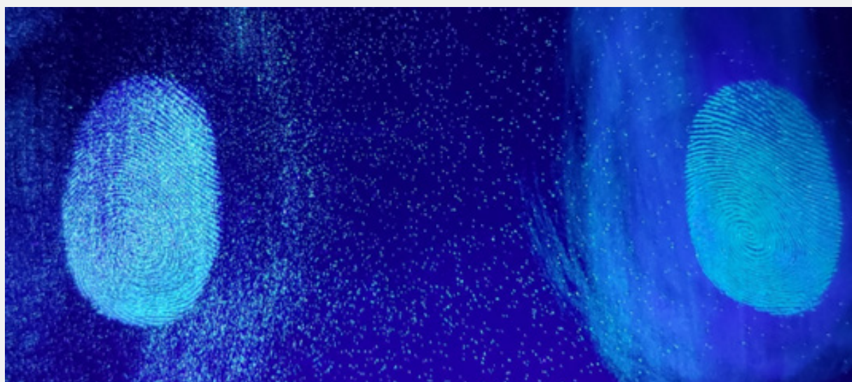
Figure 20: Fingerprints developed with phosphorescent powder (left) and with fluorescent powder (right), without using ultraviolet filter.
