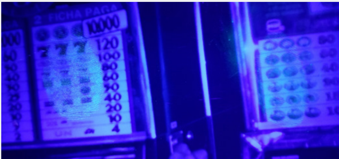
Figure 8: Prints developed with phosphorescent (left) and with green fluorescent (right), with using ultraviolet filters.
