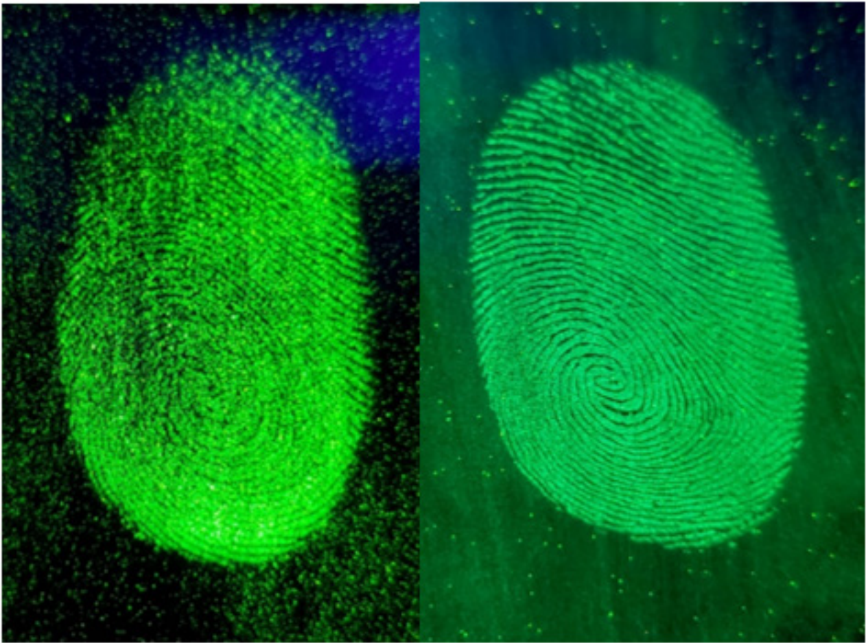
Figure 23: Comparison of fingerprint developed with phosphorescent powder (left) and fingerprint developed with fluorescent powder (right), both using ultraviolet light with filters.
