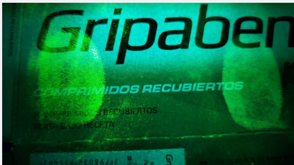
Figure 18: Fingerprints developed with phosphorescent powder (left) and with fluorescent powder (right), using ultraviolet filters.
