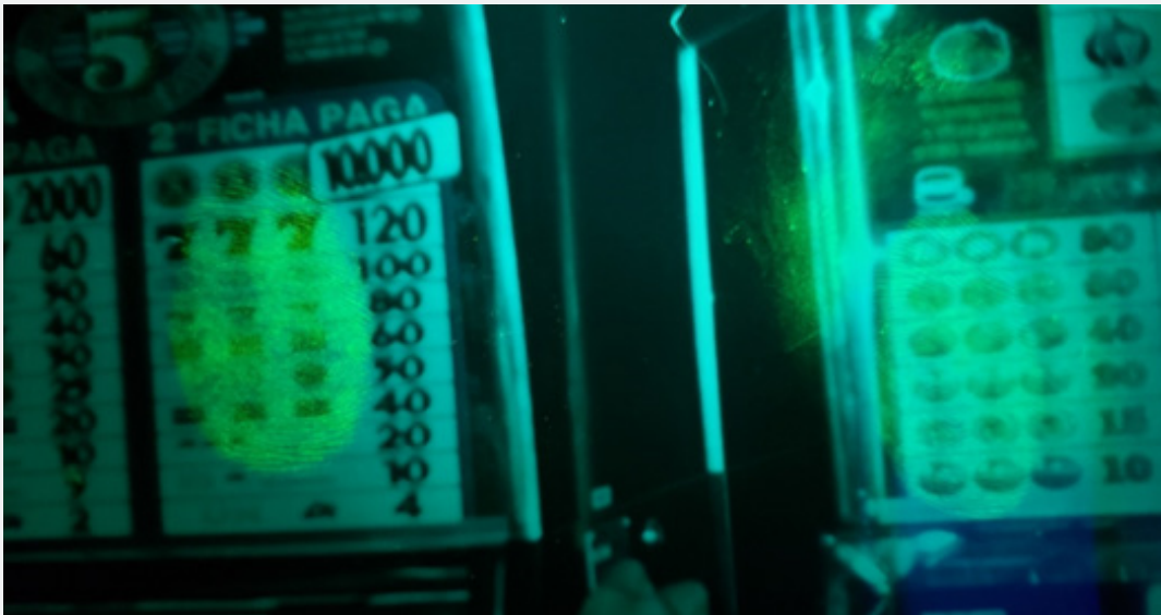
Figure 7: Prints developed with phosphorescent (left) and with green fluorescent (right), without using ultraviolet filters.
