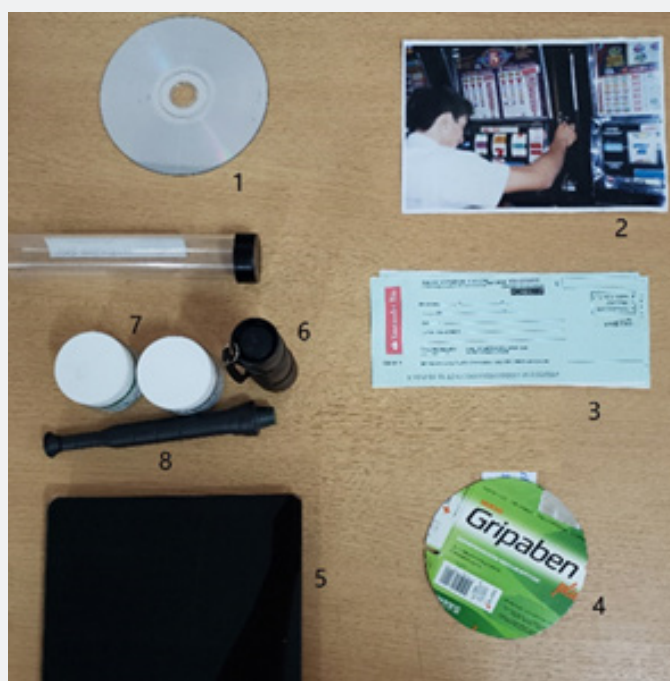
Figure 1: Illustrative image of the instruments and surfaces used: 1. CD; 2. Photograph; 3. Checks; 4. Printed cardboard; 5. Reflective glass; 6. Ultraviolet flashlight; 7. Photoluminescent powders; 8. Magnetic applicator.
